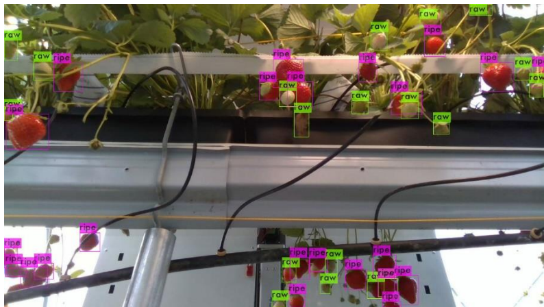
Detection network: yolo v3, 30 fps (Mask RCNN: <2 fps)
